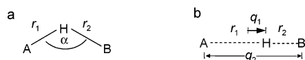
Figure 3. (a) Parameters characterizing the geometry of a hydrogen bond, i.e., the distances r_1 and r_2 and the angle ( \alpha ). (b) General hydrogen bond coordinates q_1 = 1/2(r_1 - r_2) and q_2 = r_1 + r_2 illustrated for the case of a linear hydrogen bond.
